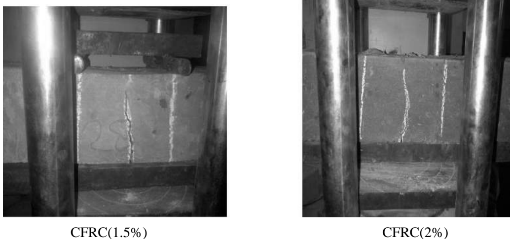
Figure 3 Crack Progression in Coconut Fibre Reinforced Concrete Beam under Flexural Loading
